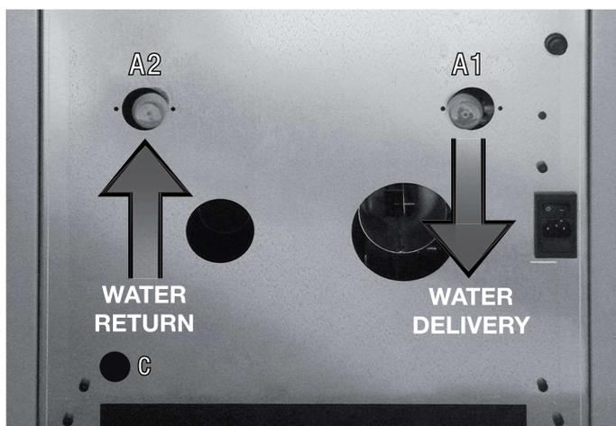
The pressure relief valve (C) must always be connected to a water drain pipe. The tube must be capable of withstanding high temperature and pressure.
