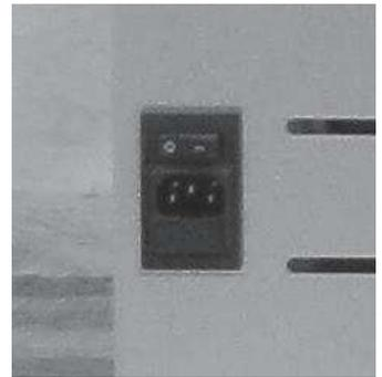
**Electrical safety:** the stove is protected against violent surges of current (ex. lightnings) by the main fuse 4 A which is located on the control panel at the rear of the thermostove. Other fuses to protect the electronic boards are to be found on the boards themselves.
