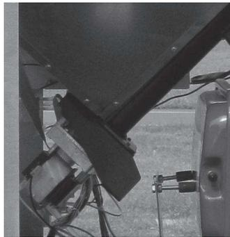
**Reduction motor:** if the motor stops, the thermostove continues to function until the flame goes out for lack of fuel, and until it has cooled down to the minimum level.
